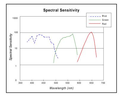
*Spectral Sensitivity:* Shows the equivalent energy needed at each wavelength in order to activate the emulsion so that it produces a neutral density of .75.
